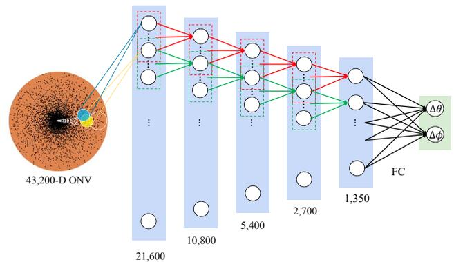
Fig. 10. The LiNet architecture. The receptive fields are depicted as circles in the retinal domain.
